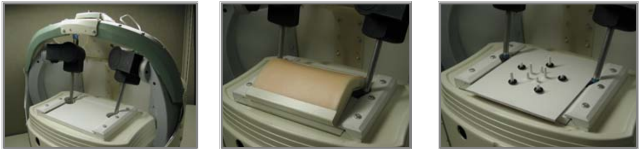
Figure 1. Front view of the CELTS system: the interface device, the railed locking and alignment mechanism, and two of the task trays are shown.
